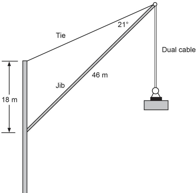
The jib is uniform, weighs 4500 kg and is 46.0 m long. The tie is a steel cable and is connected to the vertical 18.0 m above the connection of the jib, as shown in the diagram above. The angle between the tie and the jib is  $21^\circ$ .
