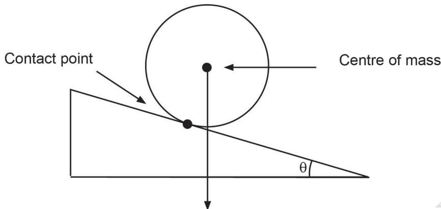
The torque about the point where a roller with mass  $m$  and radius  $r$  touches the ramp is equivalent to
