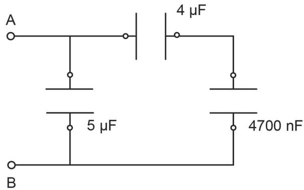
(e) Calculate the value of the capacitor required to bring the total capacitance between A and B in the circuit above to  $10 \mu\text{F}$  and correctly draw it into the circuit in part (d). (2 marks)
