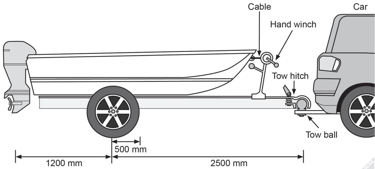
The centre of mass of the boat motor is 1.20 m behind the centre of the wheel.
