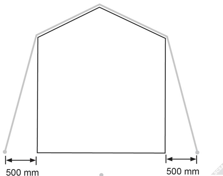
The cables are tied to pegs in the ground 500 mm from the base of the greenhouse.
